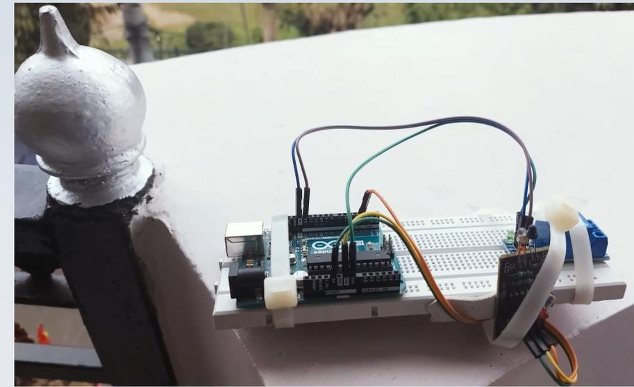
material so that the device would be affordable for most. Their prototype included an attachment that could be physically connected to an existing doorbell—converting any standard doorbell into a contactless one. If a visitor had to ring the doorbell, they would merely have to hover their hand near the button instead of pressing it.
