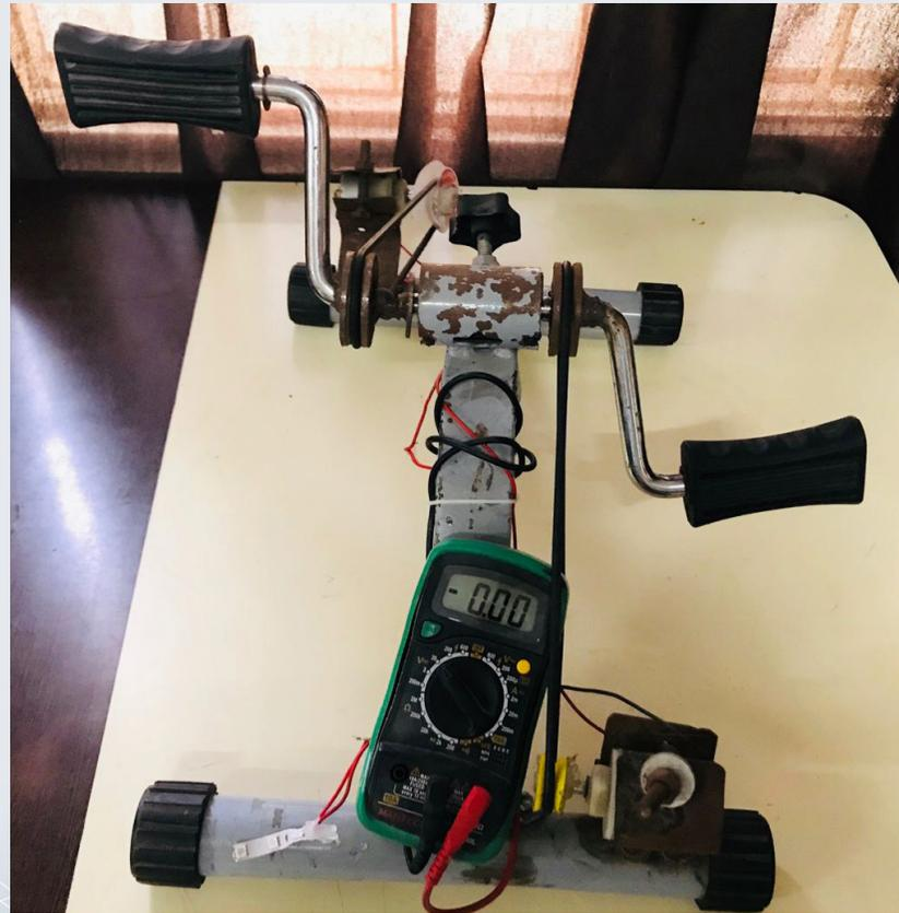
healthier lifestyle. That's how they came up with the idea of making a pedalling system to generate power. The energy generated by pedalling the device could be used for purposes like charging phones or laptops too. With the help of their mentors and the facilities available in the ATL lab, they created a prototype that was easy to pedal and simple to gauge.
