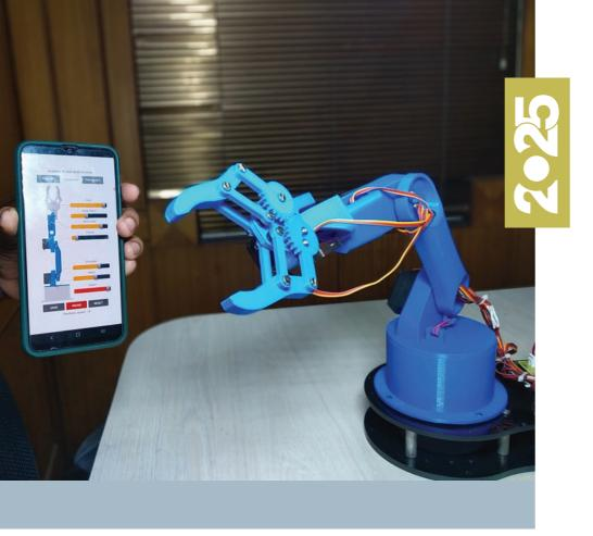
MAKE A ROTATING ROBOTIC ARM USING A SERVO MOTOR
